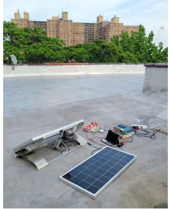
Fig. 31 Outdoor Testing Setup: This picture was taken the day before the actual test day. The tracker is in the homed position awaiting the command to start tracking.
