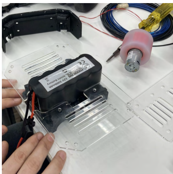
Fig. II.2. Frame assembly with layers of acrylic and motor mounts surrounding the battery.
