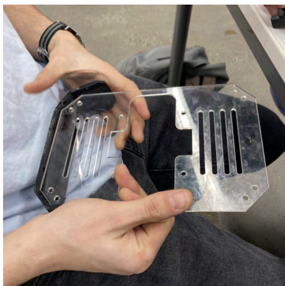
Fig. II.6. Shield wall being fit into place on the upper frame layer of acrylic.
