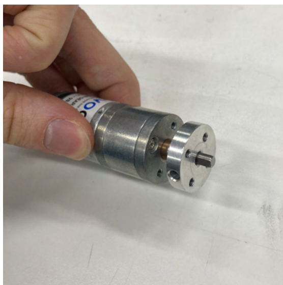
Fig. II.3. A motor hub attached to the motor axle.
