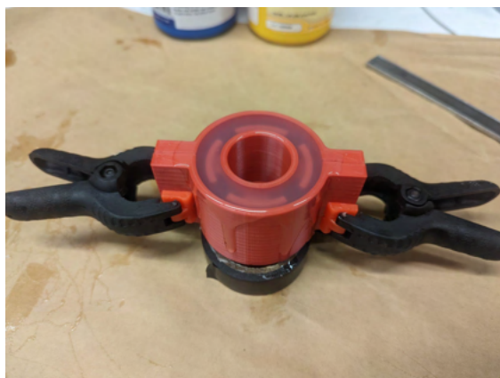
Fig. II.5. Casting process of the silicone wheels.
